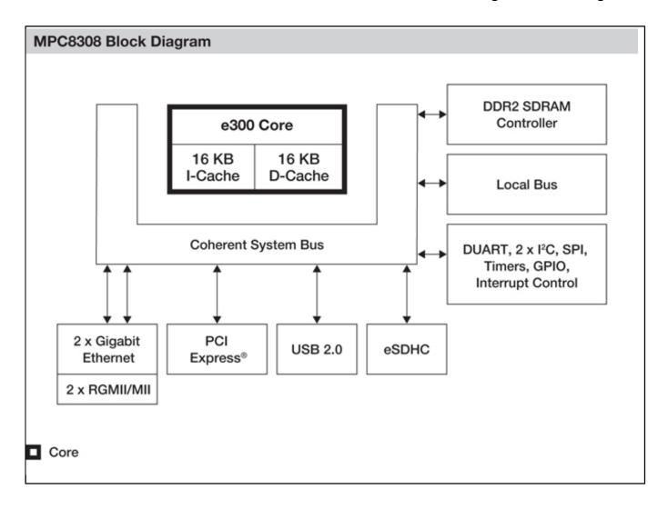
View additional information for Low-Power PowerQUICC® II Pro Processor with DDR2, eSDHC, PCI Express, eTSEC, USB, IEEE® 1588.
