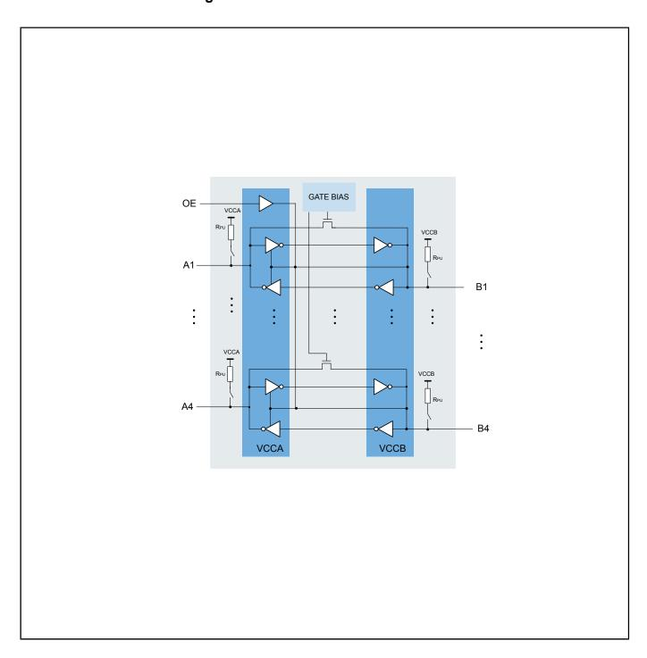
P3A1604 Typical Application Circuit Block Diagram
