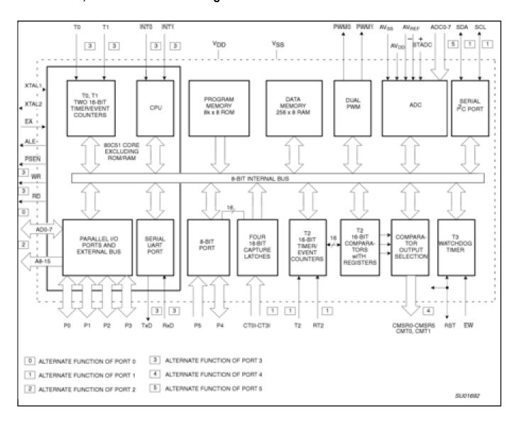
View additional information for Single-Chip 8-Bit Microcontroller with 10-Bit A/D, Capture/Compare Timer, High-Speed Outputs, PWM.
