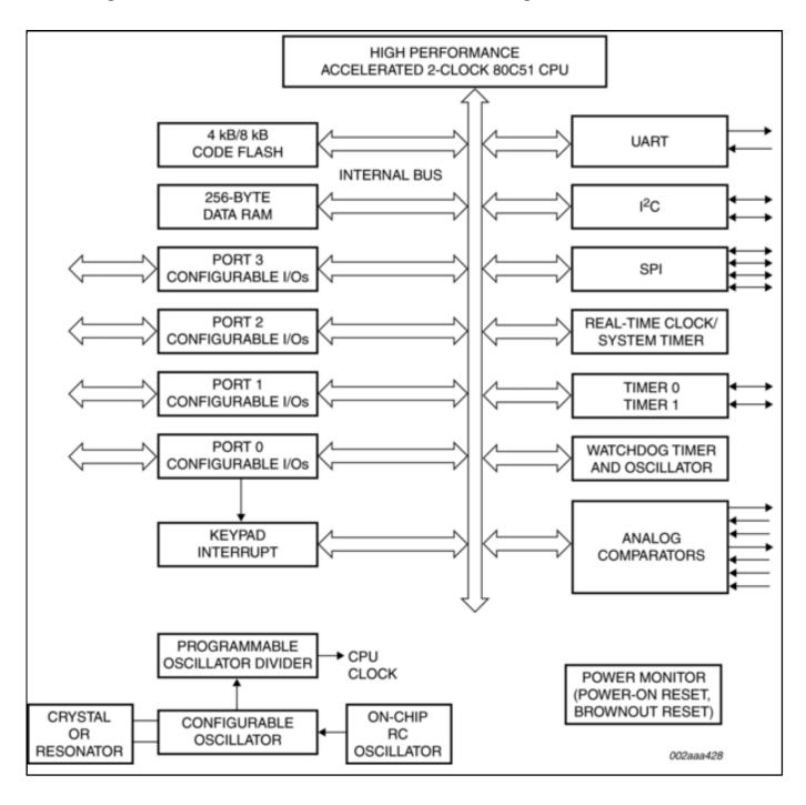
View additional information for 8-Bit Microcontrollers with Two Clock 80C51 Core 4 KB/8 KB 3 V Flash with 256 B Data RAM.
