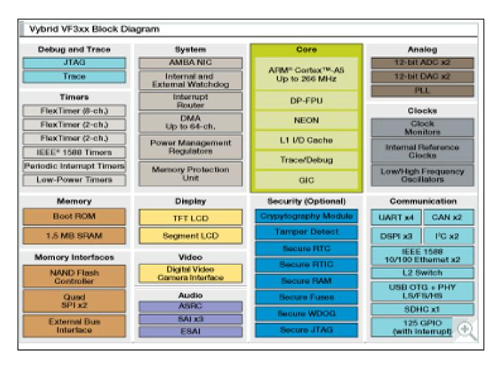
View additional information for Arm® Cortex®-A5-Based Microprocessors with 1.5MB SRAM, LCD, Security, 2x Ethernet and L2 Switch.
