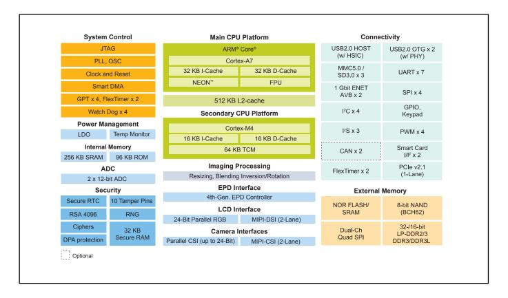
View additional information for i.MX 7Solo Processors - Heterogeneous Processing with Arm® Cortex®-A7 and Cortex-M4 Cores.
