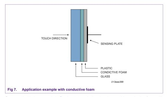
Compared with the example in <u>Section 7.1</u>, replacing the air gap with conductive foam will increase the sensitivity of the set-up.
