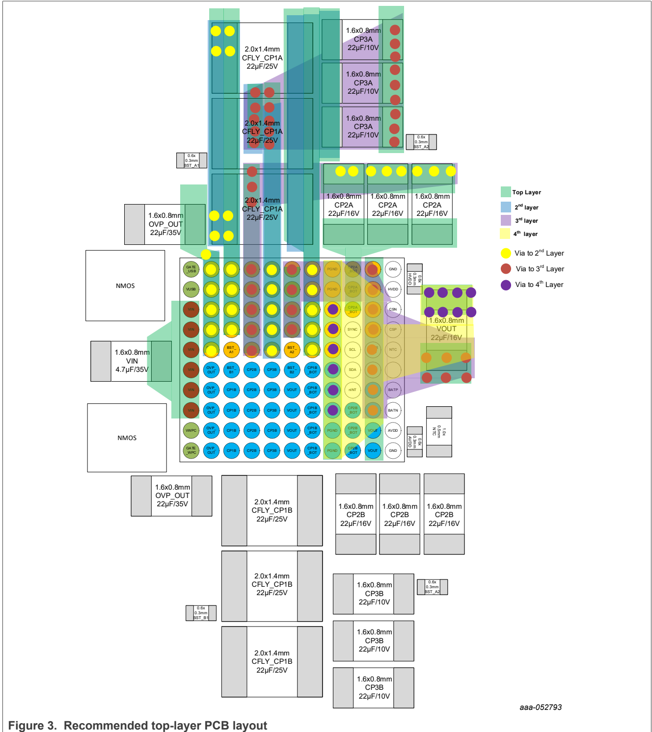
Figure 3. Recommended top-layer PCB layout
