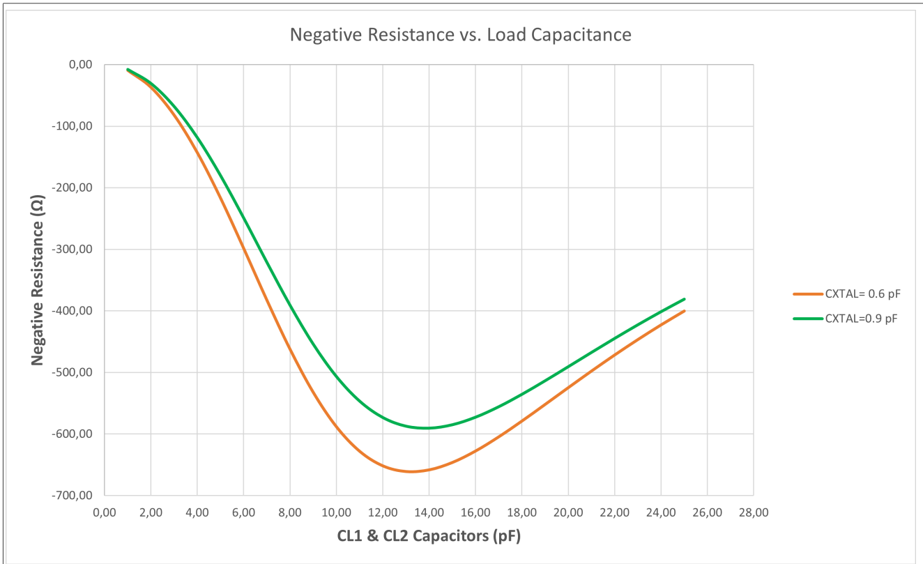
Figure 16. Negative Resistance vs. Load Capacitance, different C_{XTAL}
