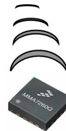
Figure 2. Linear Freefall is Defined as a Linear Translation to Earth's Surface without any Dynamic Change in Orientation
