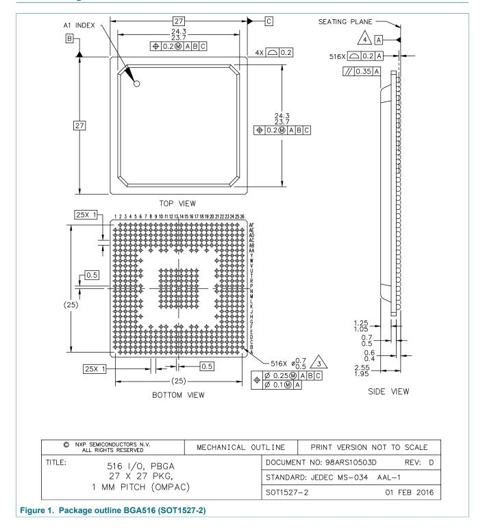
BGA516, plastic, ball grid array; 516 balls; 1 mm pitch; 27 mm x 27 mm x 1.95 mm body
