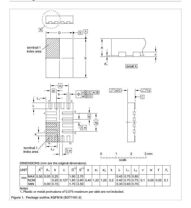
XQFN16, plastic, extremely thin quad flat package; no leads; 16 terminals; 2.6 mm x 1.8 mm x 0.50 mm
