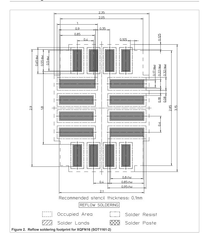
XQFN16, plastic, extremely thin quad flat package; no leads; 16 terminals; 2.6 mm x 1.8 mm x 0.50 mm
