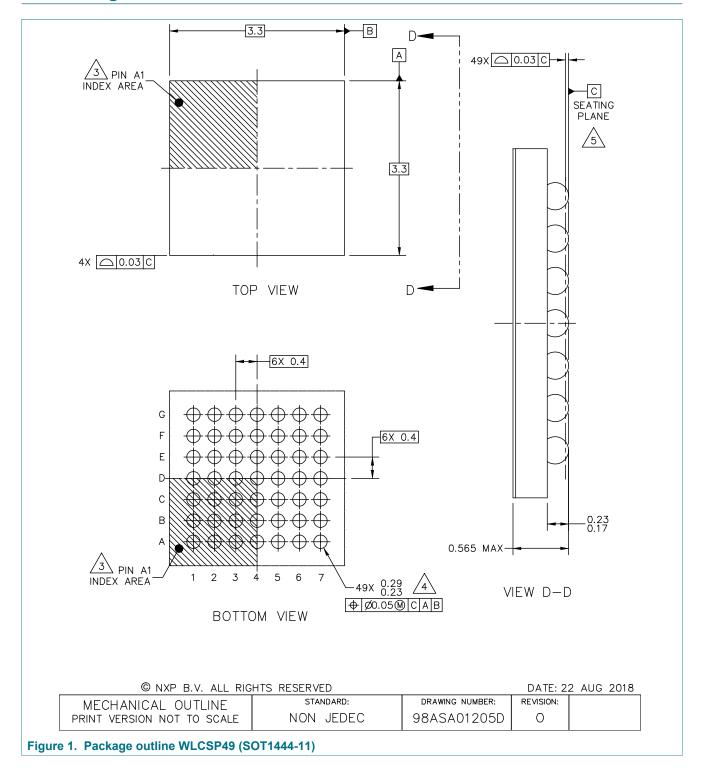
WLCSP49, wafer level chip-scale package; 49 bumps; 3.3 mm x 3.3 mm x 0.525 mm body (Backside coating included)
