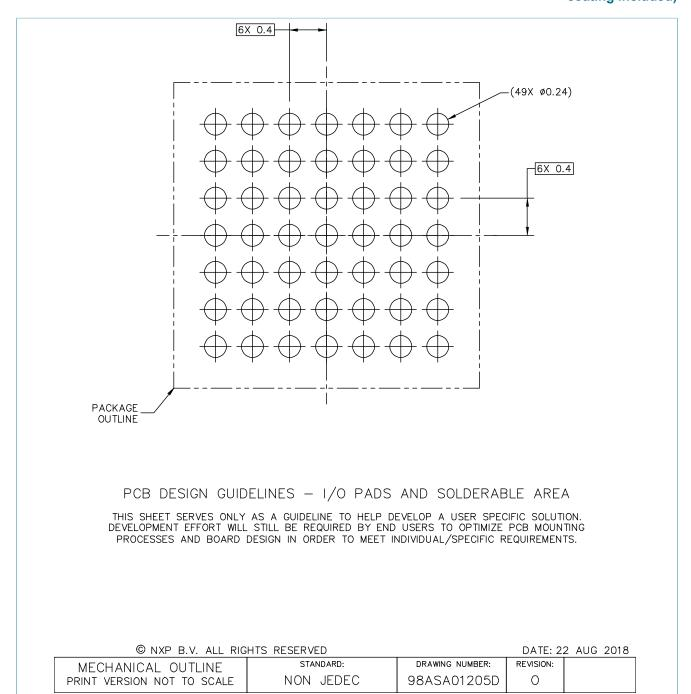
Figure 3. Reflow soldering footprint part2 for WLCSP49 (SOT1444-11)
