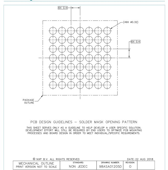
Figure 2. Reflow soldering footprint part1 for WLCSP49 (SOT1444-11)
