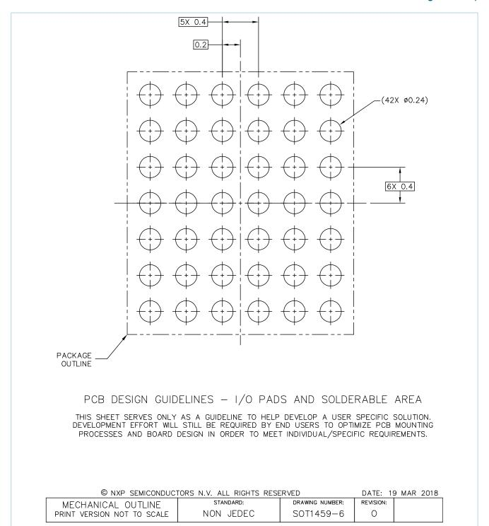
Fig. 3. Reflow soldering footprint part2 for WLCSP42 (SOT1459-6)
