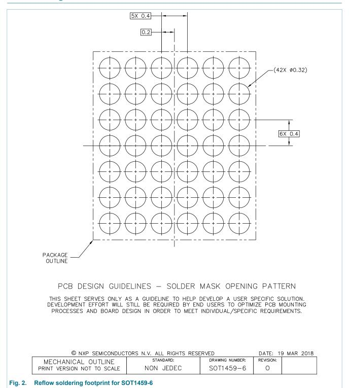
WLCSP42, wafer level chip-scale package; 42 bumps; 2.91 mm x 2.51 mm x 0.525 mm body (backside coating included)
