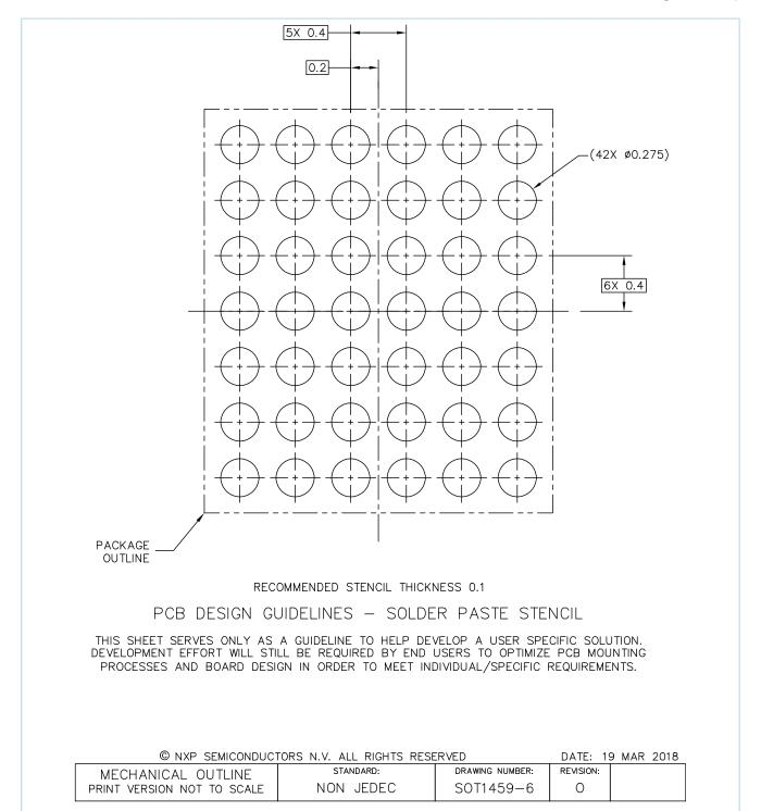
Fig. 4. Reflow soldering footprint part3 for WLCSP42 (SOT1459-6)
