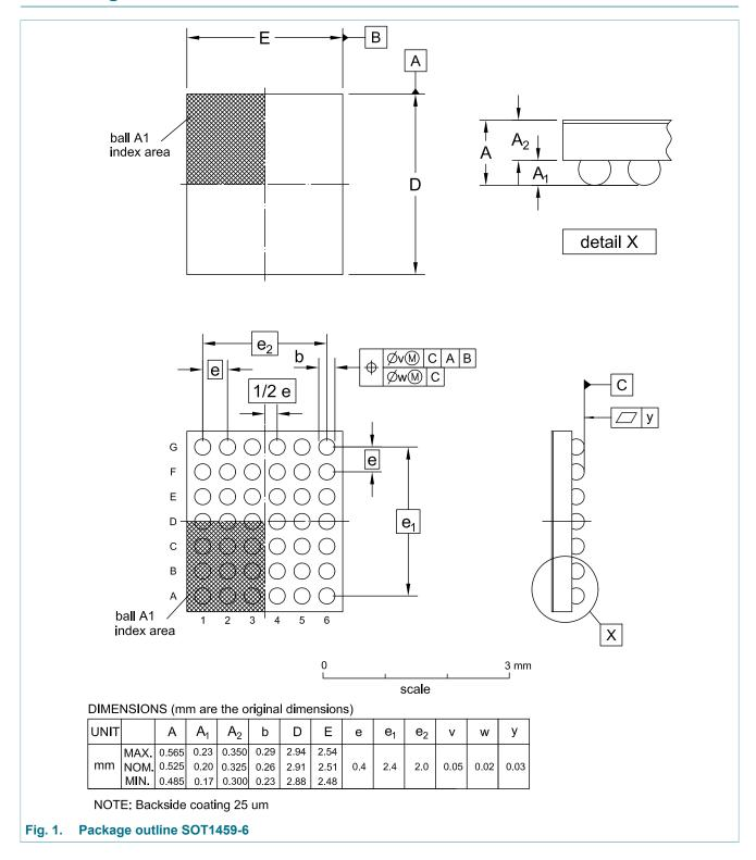
WLCSP42, wafer level chip-scale package; 42 bumps; 2.91 mm x 2.51 mm x 0.525 mm body (backside coating included)
