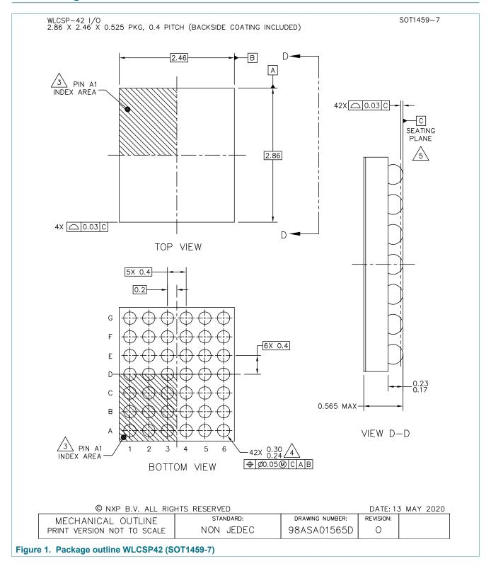
WLCSP42, wafer level chip scale package, 42 terminals, 0.4 mm pitch, 2.86 mm x 2.46 mm x 0.525 mm body (backside coating included)
