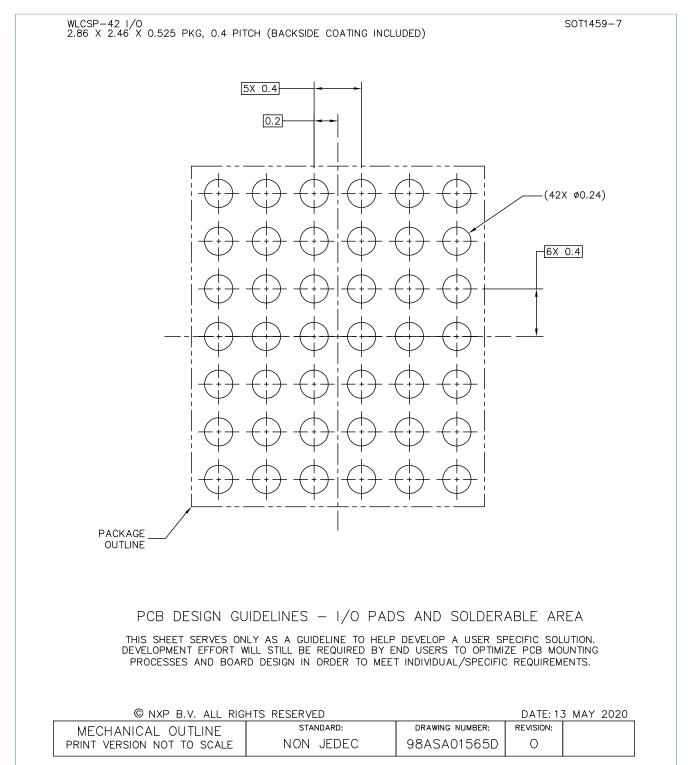
Figure 3. Reflow soldering footprint part2 for WLCSP42 (SOT1459-7)
