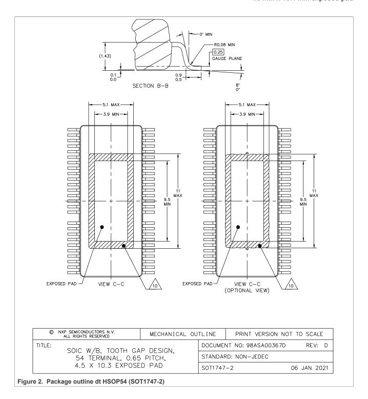
HSOP54, plastic, heatsink small outline package; W/B, tooth gap design, 54 terminals; 0.65 mm pitch; 4.6 mm x 10.4 mm exposed pad
