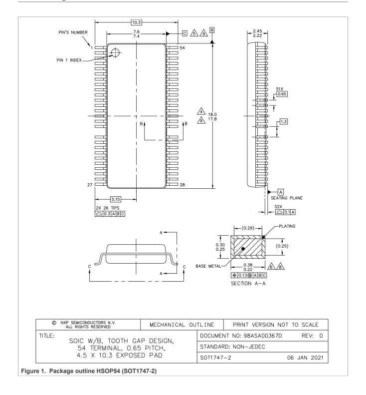
HSOP54, plastic, heatsink small outline package; W/B, tooth gap design, 54 terminals; 0.65 mm pitch; 4.6 mm x 10.4 mm exposed pad
