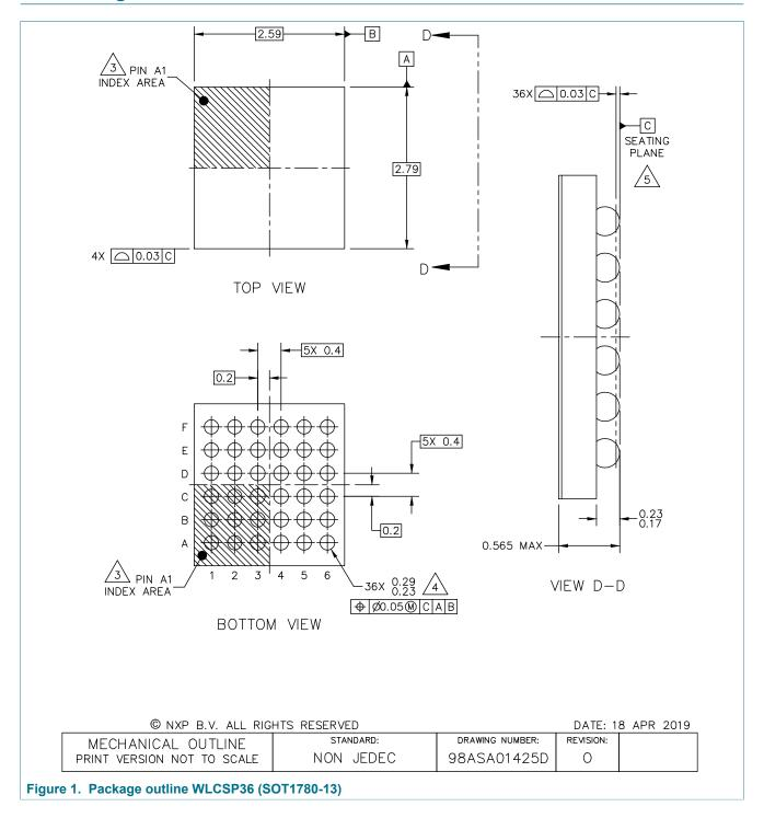
WLCSP36, wafer level chip-scale package, 36 terminals, 0.4 mm pitch, 2.79 mm x 2.59 mm x 0.525 mm body
