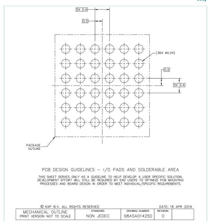
Figure 3. Reflow soldering footprint part2 for WLCSP36 (SOT1780-13)
