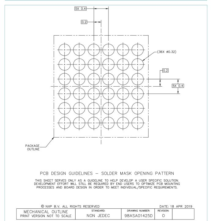
Figure 2. Reflow soldering footprint part1 for WLCSP36 (SOT1780-13)
