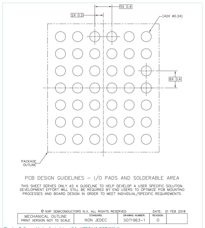
Fig. 4. Reflow soldering footprint part2 for VFBGA42 (SOT1963-1)
