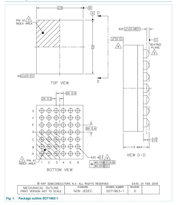
VFBGA42, plastic very thin fine-pitch ball grid array package, 42 balls, 0.4 mm pitch, 2.6 mm x 3 mm x 0.9 mm body
