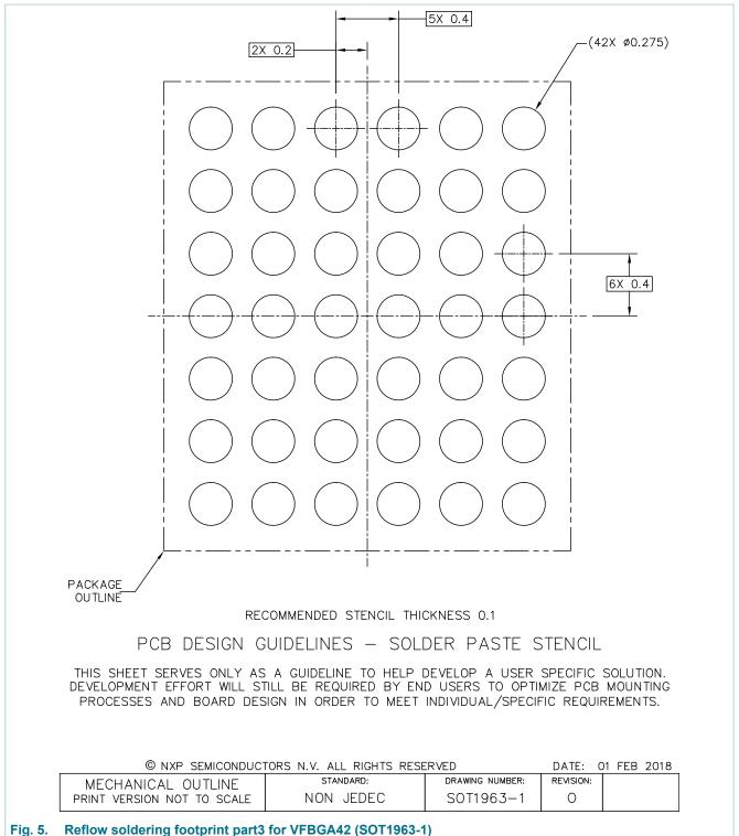
VFBGA42, plastic very thin fine-pitch ball grid array package, 42 balls, 0.4 mm pitch, 2.6 mm x 3 mm x 0.9 mm body
