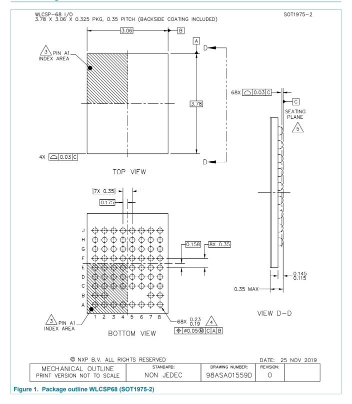
WLCSP68, wafer level chip-scale package, 68 terminals; 0.35 mm pitch, 3.78 mm x 3.06 mm x 0.325 mm body (backside coating included)
