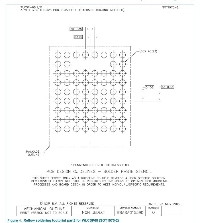
WLCSP68, wafer level chip-scale package, 68 terminals; 0.35 mm pitch, 3.78 mm x 3.06 mm x 0.325 mm body (backside coating included)
