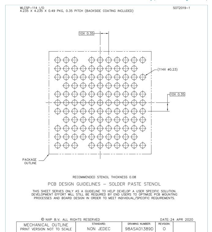
Figure 4. Reflow soldering footprint part3 for wlcsp114 (SOT2019-1)
