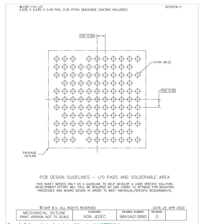
Figure 3. Reflow soldering footprint part2 for wlcsp114 (SOT2019-1)
