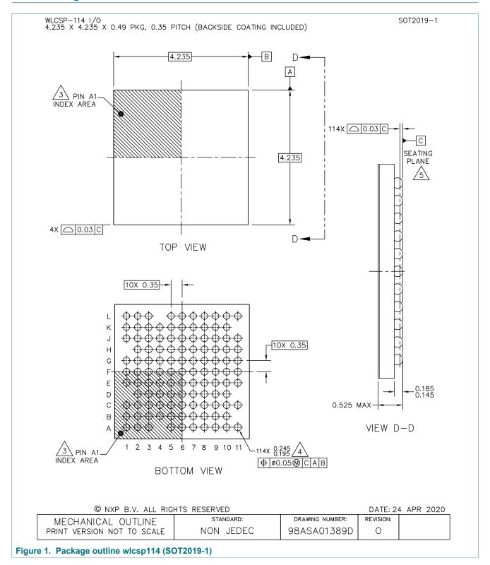
WLCSP114, wafer level chip scale package, 114 terminals, 0.35 mm pitch, 4.235 mm x 4.235 mm x 0.49 mm body (backside coating included)
