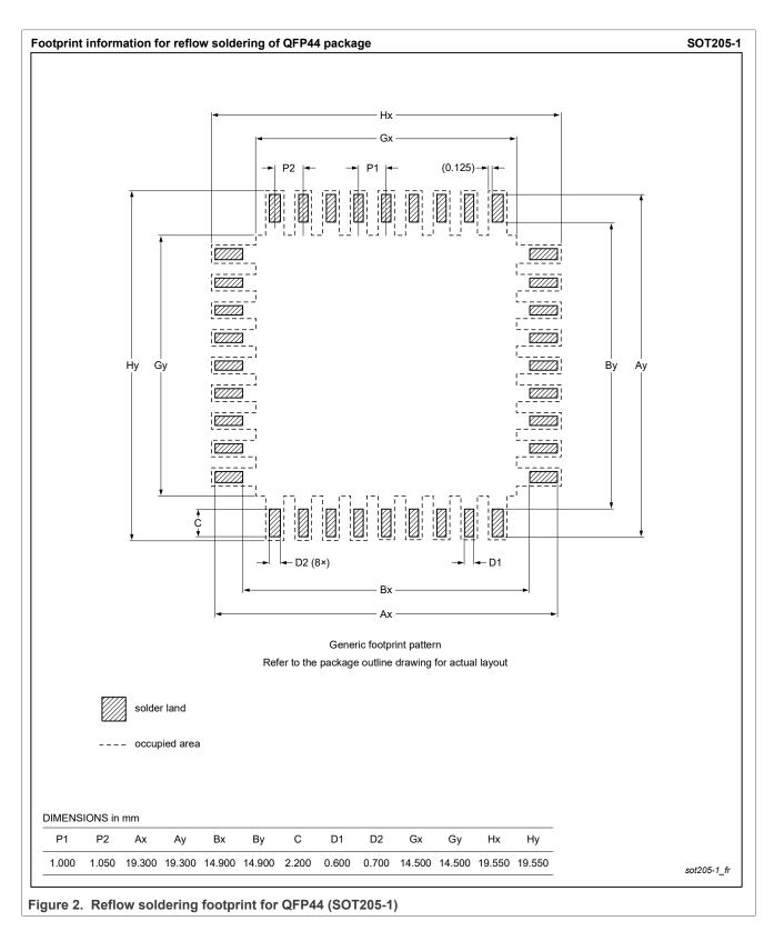
plastic quad flat package; 44 leads (lead length 2.35 mm); body 14 x 14 x 2.2 mm
