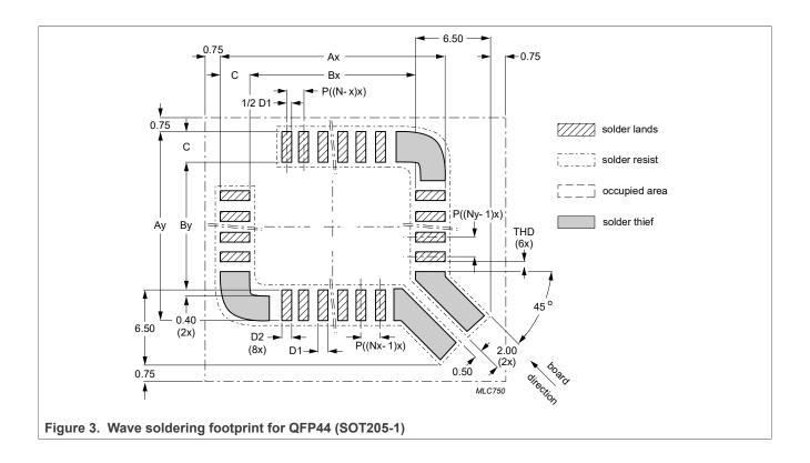
plastic quad flat package; 44 leads (lead length 2.35 mm); body 14 x 14 x 2.2 mm
