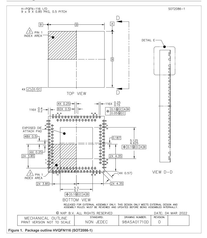
HVQFN116, thermal enhanced very thin quad flat package, no leads, 116 terminals, 0.5 mm pitch, 9 mm x 9 mm x 0.85 mm body
