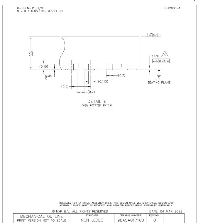
Figure 2. Package outline detail E of HVQFN116 (SOT2086-1)
