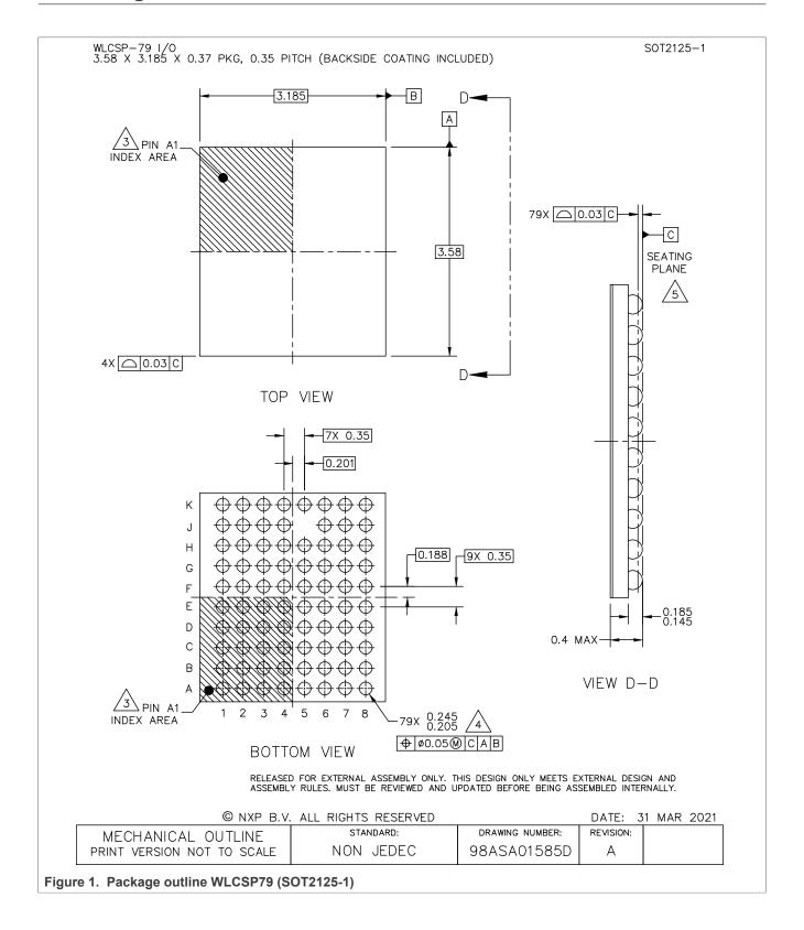
WLCSP79, wafer level chip scale package, 79 terminals, 0.35 mm pitch, 3.58 mm x 3.185 mm x 0.37 mm body (backside coating included)
