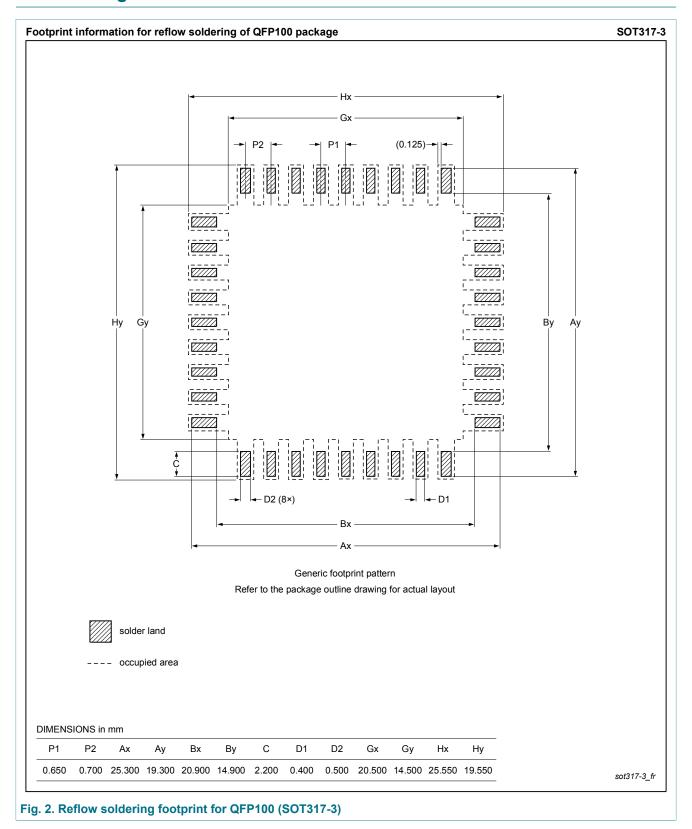
plastic quad flat package; 100 leads (lead length 1.95 mm); body 14 x 20 x 2.8 mm
