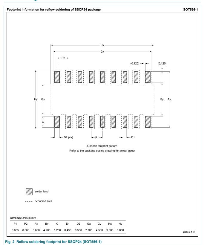
plastic shrink small outline package; 24 leads; body width 3.9 mm; lead pitch 0.635 mm
