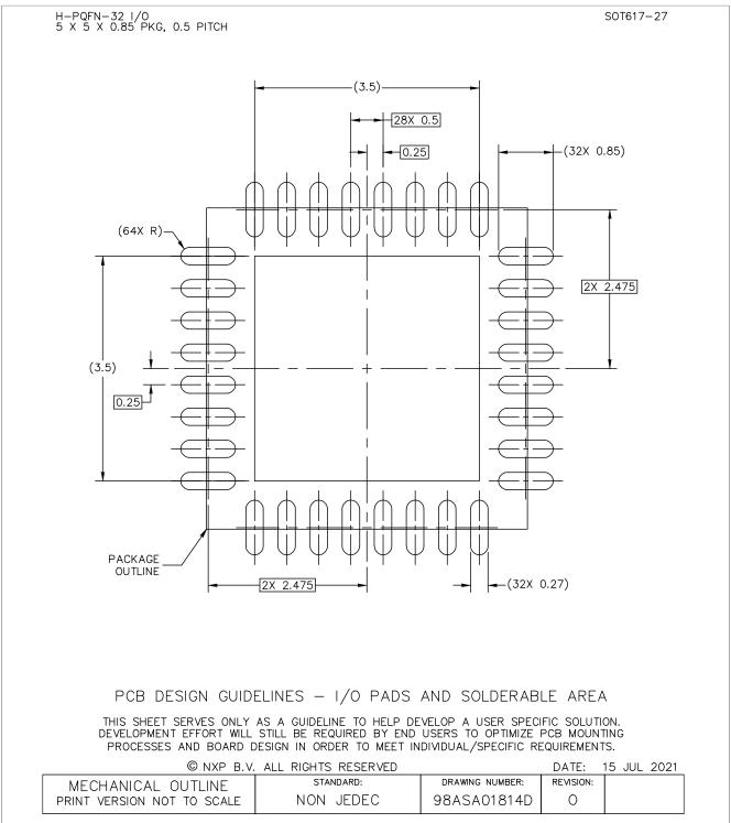
Figure 4. Reflow soldering footprint part2 for HVQFN32 (SOT617-27)
