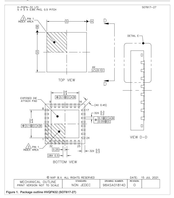
HVQFN32, plastic, thermal enhanced very thin quad flat package, no leads; 32 terminals; 0.5 mm pitch; 5 mm x 5 mm x 0.85 mm body
