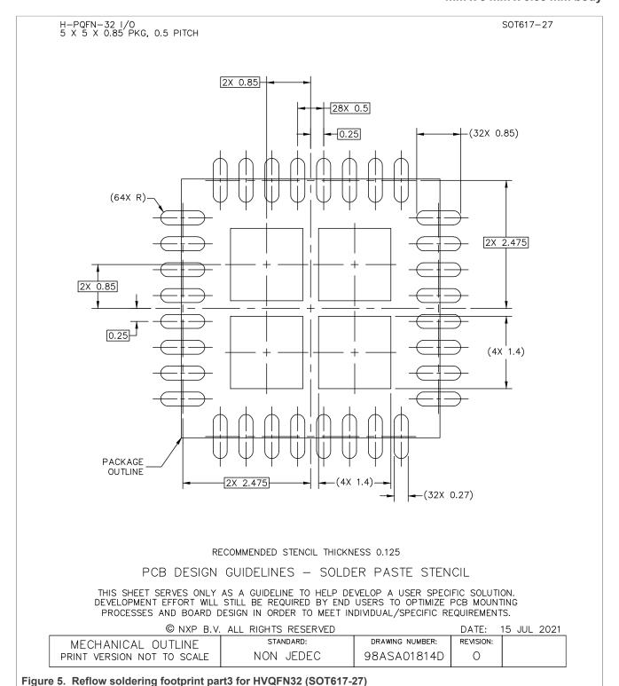
HVQFN32, plastic, thermal enhanced very thin quad flat package, no leads; 32 terminals; 0.5 mm pitch; 5 mm x 5 mm x 0.85 mm body
