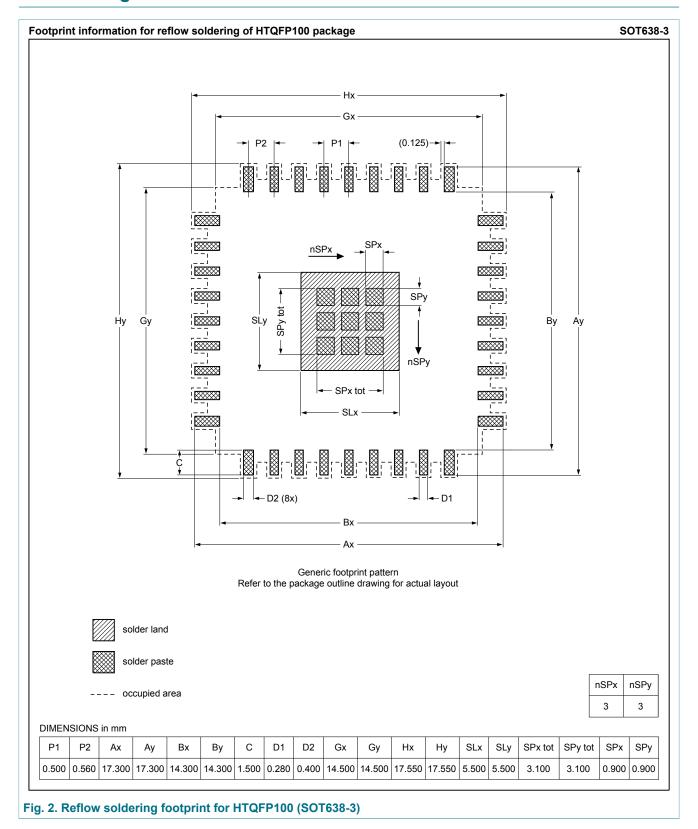
plastic thermal enhanced thin quad flat package; 100 leads; body 14 x 14 x 1 mm; exposed die pad
