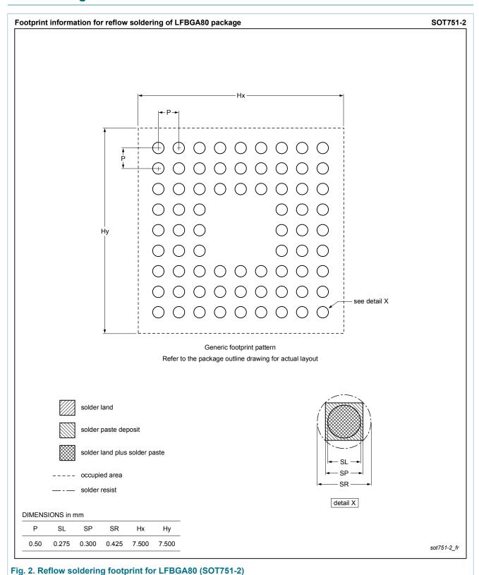
plastic low profile fine-pitch ball grid array package; 80 balls; body 7 x 7 x 0.9 mm
