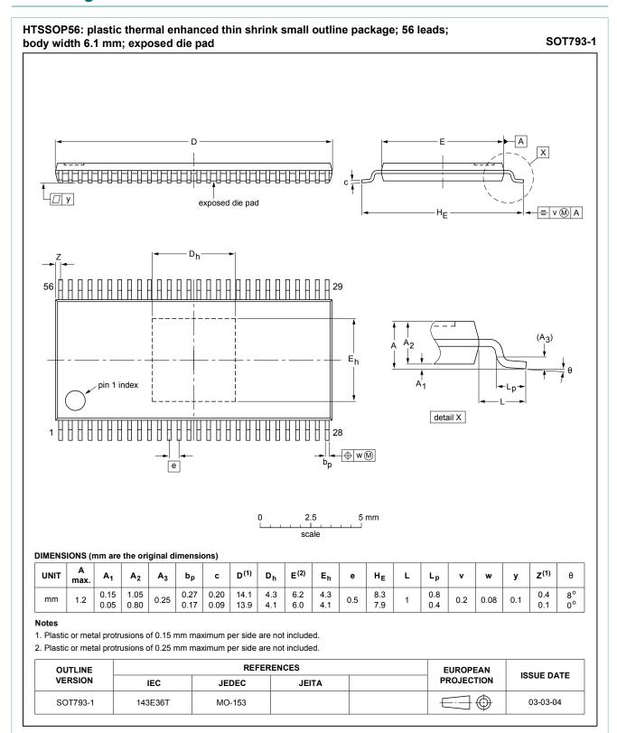
plastic thermal enhanced thin shrink small outline package; 56 leads; body width 6.1 mm; exposed die pad
