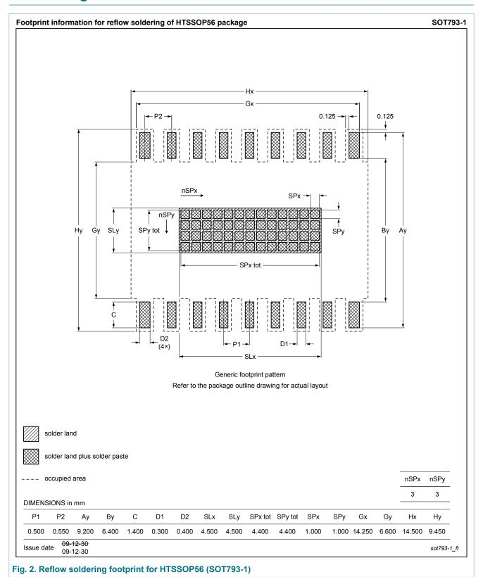
plastic thermal enhanced thin shrink small outline package; 56 leads; body width 6.1 mm; exposed die pad
