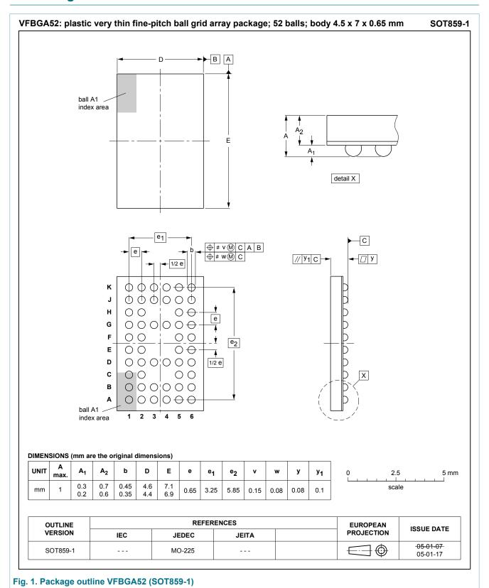
plastic very thin fine-pitch ball grid array package; 52 balls; body 4.5 x 7 x 0.65 mm
