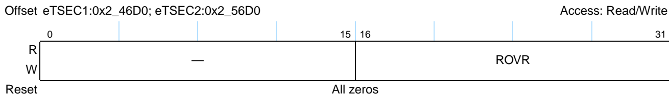
Figure 15-72. Receive Oversize Packet Counter Register Definition
