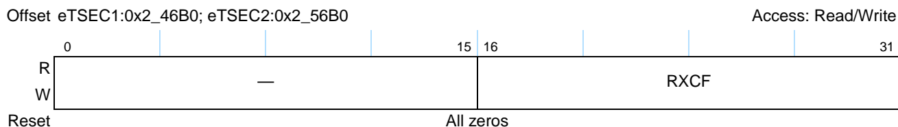
Figure 15-64. Receive Control Frame Packet Counter Register Definition
