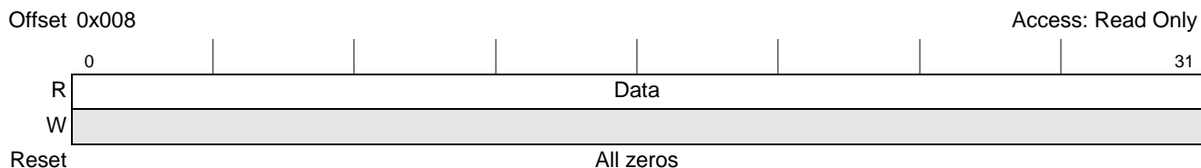
Figure 17-5. PCI INT_ACK Register
