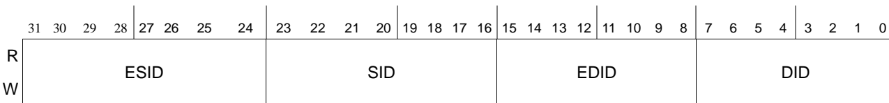
Figure 16-47. Inbound Block m Type8 Classification n Rule Mask Register 0 (IB m T8C n RMR0)
