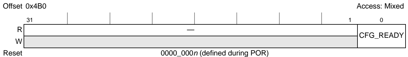
Figure 17-140. PCI Express Configuration Ready Register (PEX_CFG_READY)
