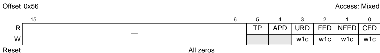
Figure 17-104. PCI Express Device Status Register
