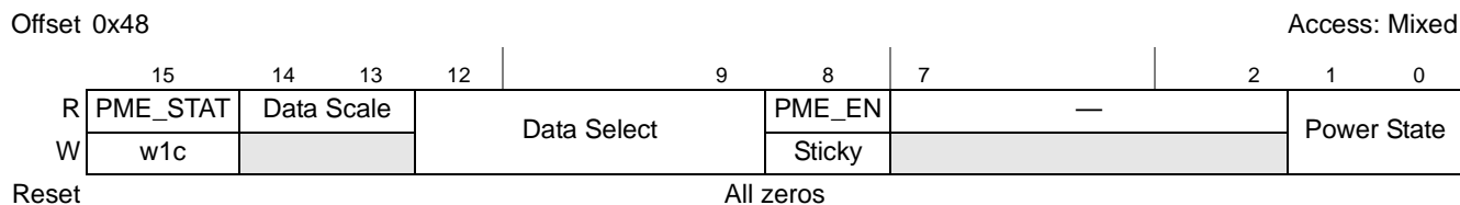
Figure 17-98. PCI Express Power Management Status and Control Register
