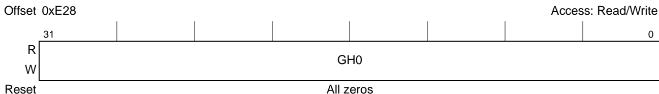
Figure 17-46. PCI Express Error Capture Register 0 (PEX_ERR_CAP_R0) External Source, Inbound Transaction
