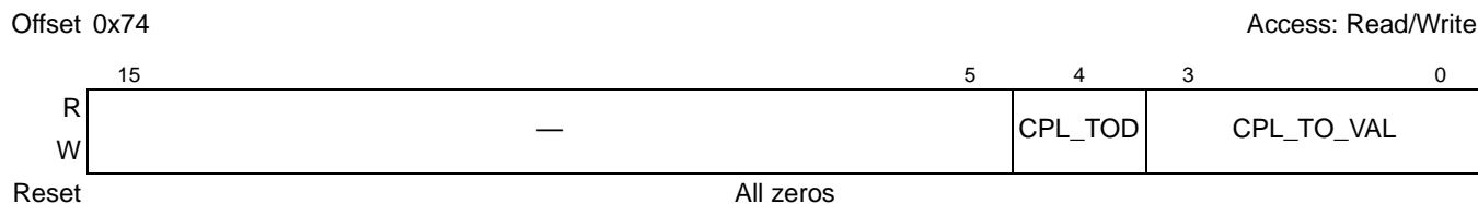
Figure 17-114. PCI Express Device Control 2 Register
