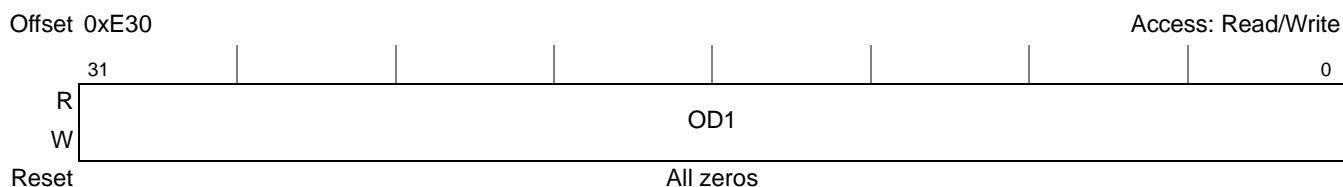
Figure 17-49. PCI Express Error Capture Register 2 (PEX_ERR_CAP_R2) Internal Source, Outbound Transaction
