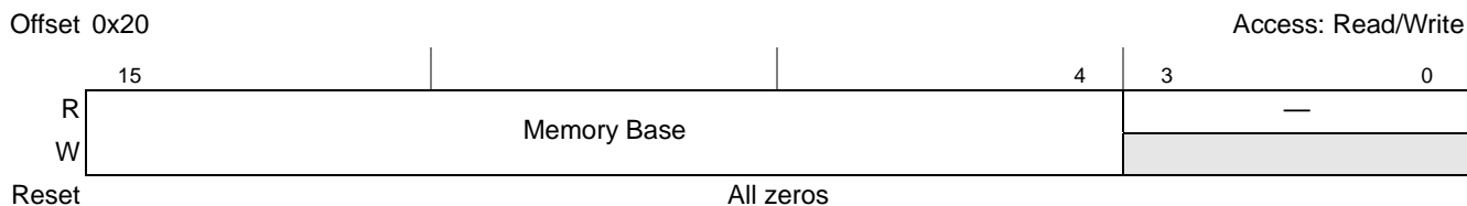
Figure 17-83. PCI Express Memory Base Register
