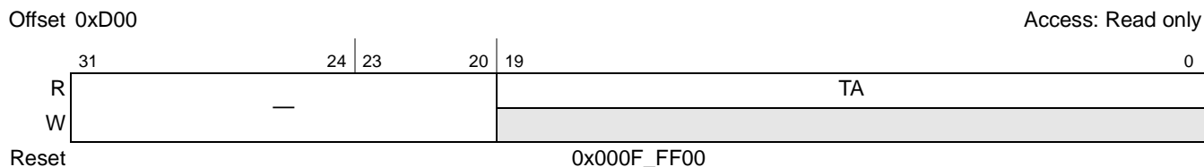
Figure 17-37. PCI Express MSI Inbound Translation Address Register (PEXMSIITAR)
