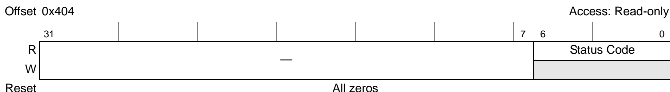
Figure 17-135. PCI Express LTSSM State Status Register (PEX_LTSSM_STAT)
