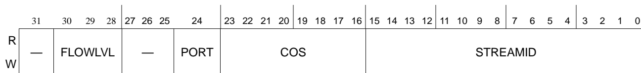
Figure 16-55. Inbound Block m Type9 Classification n Rule Value Register 1 (IB m T9C n RVR1)
