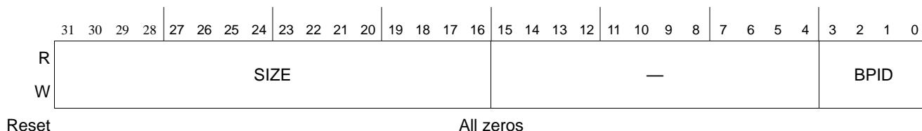
Figure 16-49. Inbound Block m Type8 Classification n Data Buffer Pool Register (IB m T8C n DBPR)
