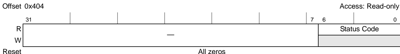
Figure 17-135. PCI Express LTSSM State Status Register (PEX_LTSSM_STAT)
