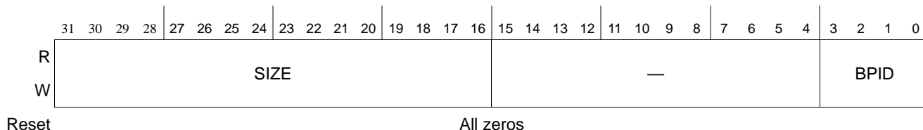
Figure 16-69. Inbound Block m Type10 Classification n Data Buffer Pool Register (IBmT10CnDBPR)
