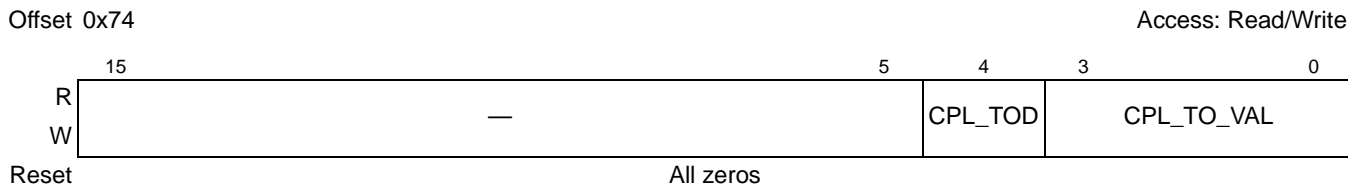
Figure 17-114. PCI Express Device Control 2 Register
