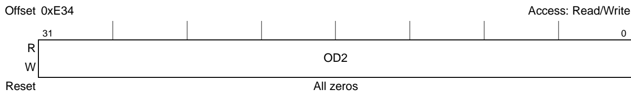
Figure 17-51. PCI Express Error Capture Register 3 (PEX_ERR_CAP_R3) Internal Source, Outbound Transaction
