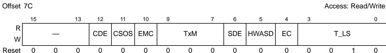
Figure 17-115. PCI Express Link Control 2 Register
