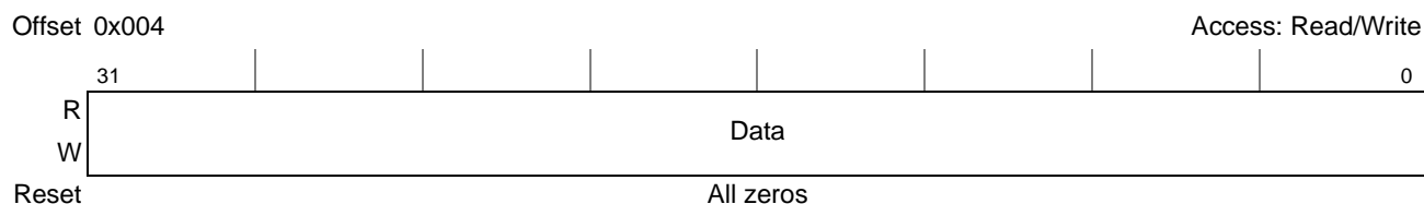
Figure 17-13. PCI Express Configuration Data Register (PEX_CONFIG_DATA)
