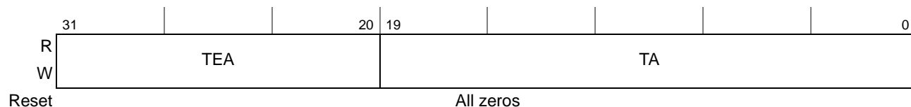
Figure 17-29. PCI Express Outbound Translation Address Registers (PEXOTAR n )
