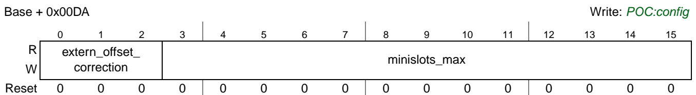
Figure 29-100. Protocol Configuration Register 29 (FR_PCR29)
