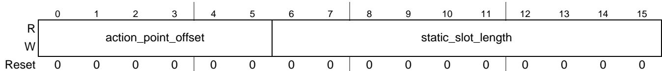
Figure 29-71. Protocol Configuration Register 0 (FR_PCR0)
