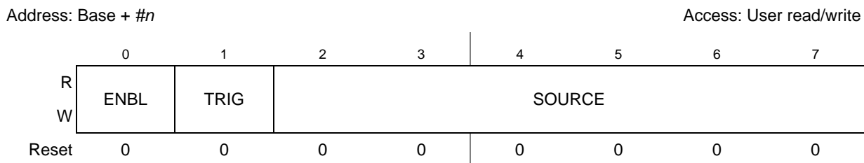
Figure 20-2. Channel Configuration Registers (CHCONFIG#n)
