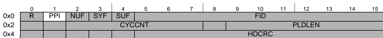
Figure 29-124. Frame Header Structure (Transmit Message Buffer for Key Slot)
