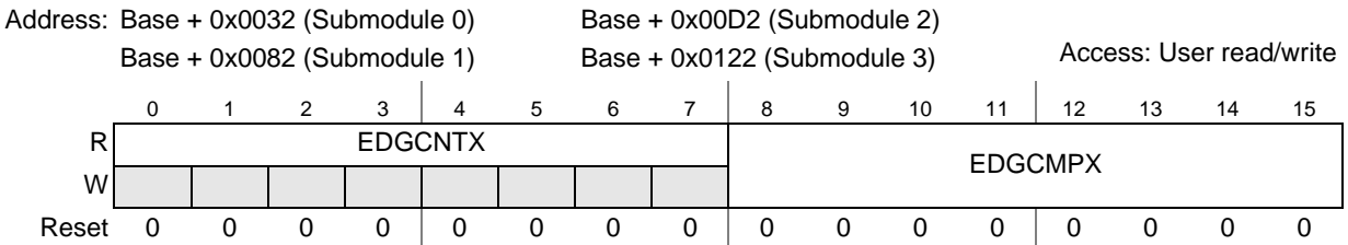
Figure 28-22. Capture Compare X register (CAPTCMPX)
