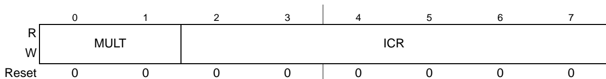
Figure 31-4. I 2 C Bus Frequency Divider Register (IBFD)
