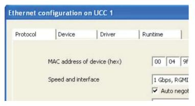
The block configuration box is broken down to three types—protocol, device and driver. Another tab is available for runtime control when relevant
