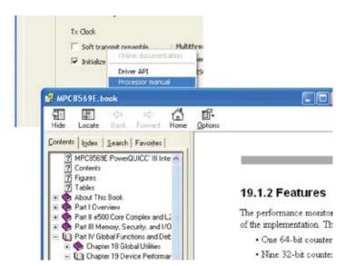
Sometimes the full specification is needed—right click the field to gain immediate, pin-pointed access to the relevant manual of your choice
