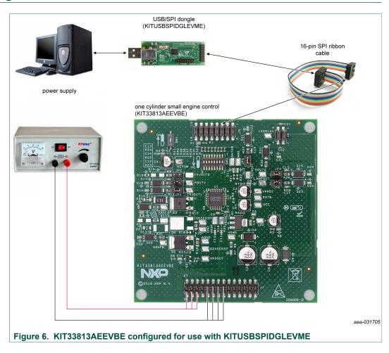
To perform the examples included in the software bundle, the following connections and setup must be performed:
