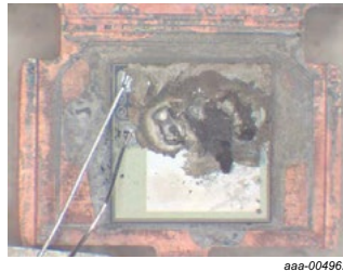
Fig 76. Sample image 4: source wires fused
