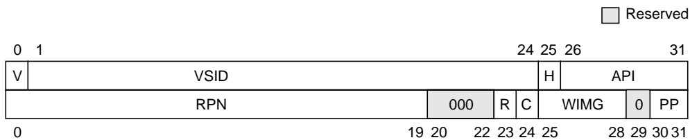
Figure 7-22. Page Table Entry Format—32-Bit Implementations
