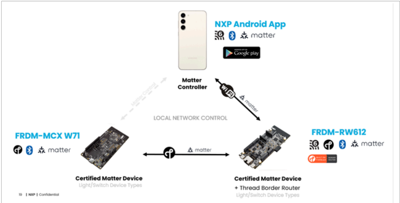
Figure 2. Matter applications based on NXP CHIP Tool App, FRDM- RW612 and FRDM-MCXW71
