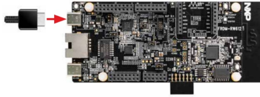
Figure 6. Connect the FRDM-RW612 board to a PC using the USB Type-C® cable
