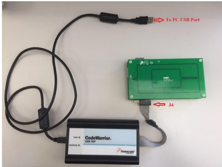
Figure 30. Connecting the debug cable to the board
